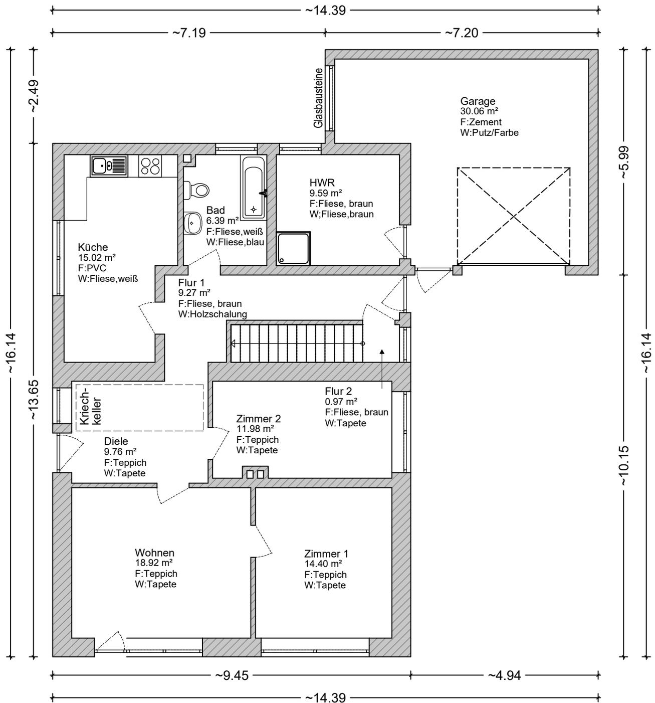
GRUNDRISS ERDGESCHOSS M = 1:100
