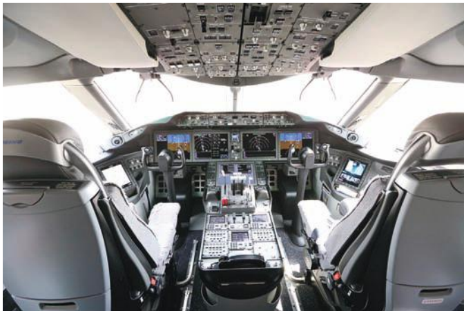
Figure 1.1 Measuring instruments on the flight deck of a passenger jet provide the crew with information about the performance of the aircraft.
