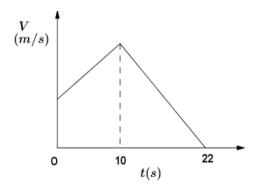
The diagram is a velocity-time graph of an object which accelerated uniformly for 10 seconds. During this time the velocity, V m/s at time t seconds from the start, was given by V=6+2t. It then decelerated to rest in a further 12 seconds.
