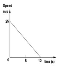
The graph show the motion of a car which decelerates uniformly from a speed of  $25~\mathrm{m/s}$  until it come to rest in  $10~\mathrm{seconds}$ .
