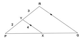
In the diagram, XY is parallel to QR, PY = 2 cm, YR = 3 cm and XY = 4 cm
