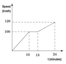
The diagran shows part of a speed-time graph of a car. The car starts from rest and accelerates uniformly to a speed of  $100~\rm km/h$  in  $10~\rm minutes$ . It maintains that speed for 3 minutes and then accelerates uniformly for a further 11 minutes until it reaches a speed of  $120~\rm km/h$ .
