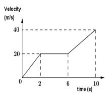
The diagram is the velocity-time graph of an object which accelerates uniformly from rest and attains a velocity of 20 m/s in 2s. The object maintains a constant velocity for a further 4s and then accelerates uniformly again for 4s after which it reaches a velocity of 40 m/s.
