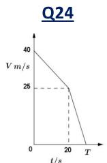
The diagram shows a velocity-time graph of a particle which decelerates uniformly from a velocity of 40 m/s to a velocity of 25 m/s in 20 seconds. It further decelerates uniformly at a rate of 2,5 m/s $^2$  until it comes to rest.
