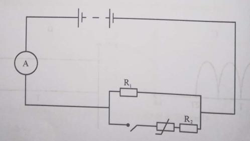
When the switch is closed, the ammeter reading is 3.0 A with the thermistor at 20 °C. How would the ammeter reading change when the temperature changes to 40 °C?
