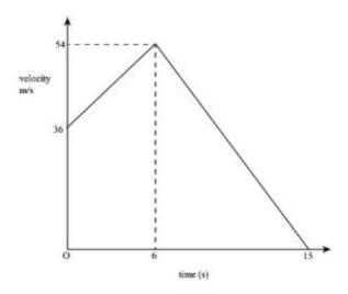
The diagram shows the velocity-time graph of a moving object which accelerates uniformly from 36 m/s to a velocity of 54 m/s in 6 seconds. It then retards uniformly to rest in a further 9 seconds.
