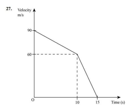
The diagram is the velocity – time graph of an object which decelerates uniformly from a velocity of 90 m/s to a velocity of 60 m/s in 10 seconds. It then decelerates uniformly to rest in a further 5 seconds.
