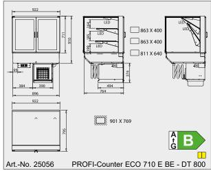
The drawings are shown with special accessory that is not included. The PROFI-Counter 1200s display cases are equipped with sliding doors on the operator side and 40 cm longer. (External dimensions are identical to the refrigerated display case Euro-Counter E BE 1200 and Euro-Counter ECO E BE 1200)
