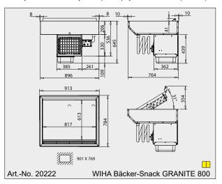
The exterior is made of galvanised sheet steel. Inside the pan is a generously sized circulating air evaporator with coated surface and quiet low-voltage ventilators (12 V DC) for air circulation.
