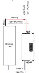
Wiring with non-dimming ballast or LED driver. Non-Dimming Driver
