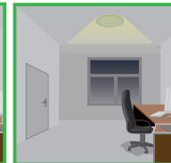
The light still dims to 0/10%/30%/50% if still insufficient natural light, the light never switches off until sufficient natural light.
