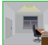
If with insufficient natural light, the light automatically dims to 0, 10%, 30%, 50%.
