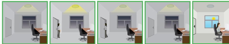
If with insufficient natural light, the light automatically dims to 0, 10%, 30%, 50%.
