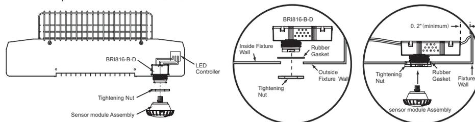
Note: The Outside Fixture Wall thickness should be no greater than 0.125" (3.18mm) for optimal sensor mounting and security.
