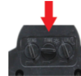
Motion sensor has adjustments for motion sensitivity, time delay, and photo control
