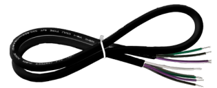
SCL-12FT-SJTW18/6-BK BLACK 12 FT. CORD, SJTW 18 AWG 6-CONDUCT ( WH/BK/GN/PU/GY + RED FOR EMERGENCY)
