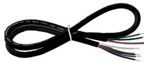
SCL-12FT-SJTW18/5-BK BLACK 12 FT. CORD, SJTW 18 AWG 5-CONDUCT ( WH/BK/GN/PU/GY)
