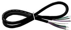
SCL-6FT-SJTW18/6-BK WHITE 6 FT. CORD, SJTW 18 AWG 6-CONDUCT ( WH/BK/GN/PU/GY + RED FOR EMERGENCY)
