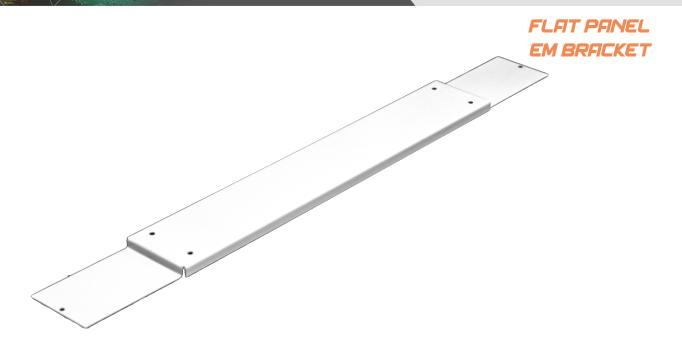
**LP-EMMB** is a 2-Foot painted steel mounting bracket for easy mounting of emergency backup units on top of 2X2 and 2X4 flat panel lights. Use it with Westgate Controls **ELB-2048-EXTR** emergency unit or any other brand. If hole patterns don't match your EM unit of choice, use self-tapping screws to position and mount your unit.
