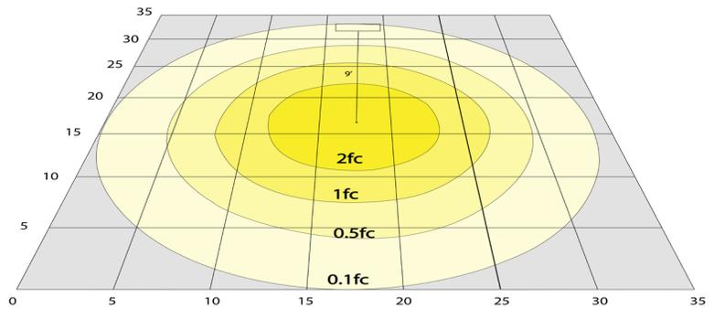
Simulation Based on 2700K Area 30'x30' Mounting Height: 9'
