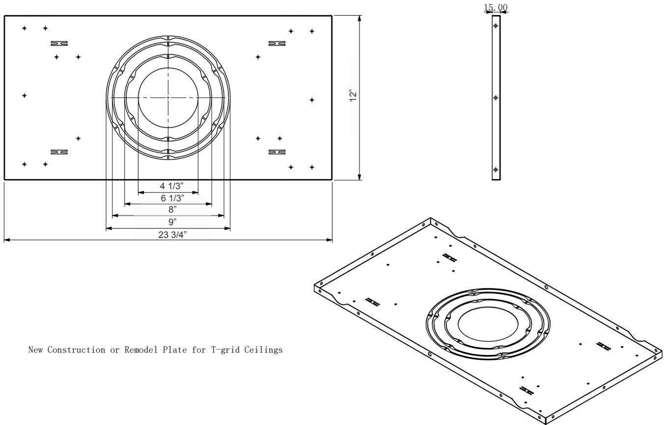
New Construction or Remodel Plate for T-grid Ceilings
