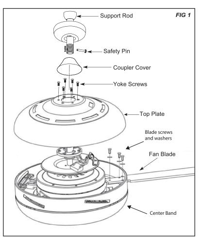
Back off (loosen) the set screws (2) in the support rod coupler until the inside of the channel is clear of the screw tip. Remove and save the safety pin and washer on the end of the support rod assembly. Slide the ceiling canopy onto the support rod, followed by the support rod coupler cover (see *figure 1*). Feed the electrical wires from the fan housing through the support rod.
