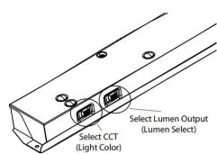
5.Remove driver box from package and use switch to select appropri-ate light color (CCT) and light output (lumen).
