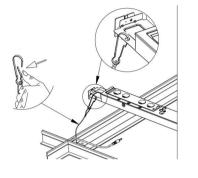
10. Secure luminaire to driver box by attaching tether cable from luminaire to opening on the driver box using clip.
