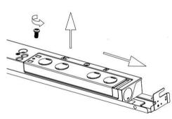
7.Remove driver box access plate by removing screw from driver box cover and locate the driver supply wire (1 black, 1 white, 1 green /ground).
