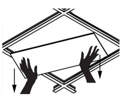
1.Remove original ceiling tile from the T-Grid ceiling.
