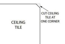
2.Cut out one corner of the ceiling tile using the provided template.
