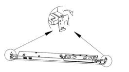
6. Rotate the buckle 90° clockwise.
