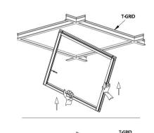
4.Install luminaire to the opening in the T-Grid by raising the luminaire above the grid, then lower it until it rests between the T-Grid and the tile opening. Cable side of the luminaire must align with cable side of the driver box.
