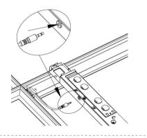
11. The DC cable of the lamp body is connected to the power supply
