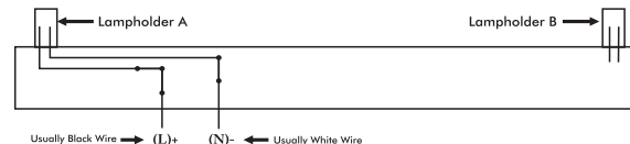
Figure 6: These LED tubes can retrofit maximum four lamps in one luminaire. The revised circuit diagram as shown in Fig.3. Please see Fig.2 and Fig. 5 to cut wires and to connect wires as follows:
