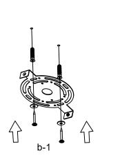
B. Secure the backplate of canopy using anchor, washer and screws.
