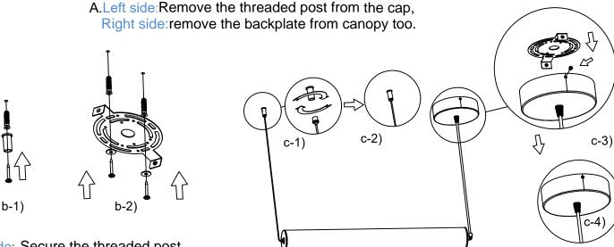
B.Left side: Secure the threaded post using anchor and screws.
