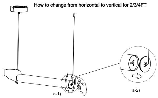
A.Hold the housing with one hand and unscrew the end cap with the aircraft cable using the other hand.
