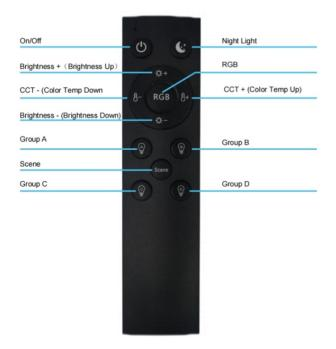
Reset Time: on/off between 1 second for 5 times
