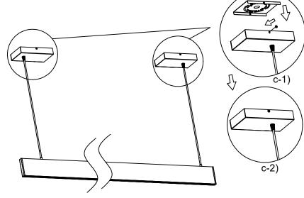
C.Install the electrical box to the ceiling cover plate.
