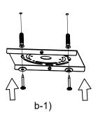
B.Fix the electrical box cover with ceiling screws.
