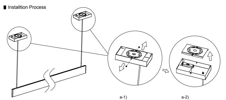
A.Remove the back cover of the power supply box. (Two drive boxes on 8FT)
