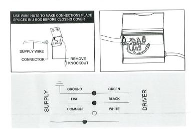
Step4: Secure the junction box to the frame plate .
