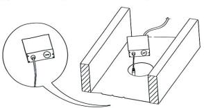
Step 5: Connect downlight to junction box powercord & install.
