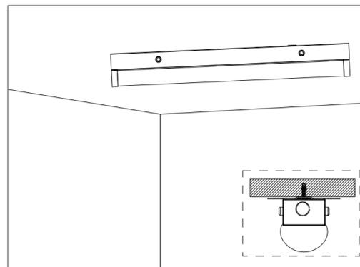
1. Punch a hole on the wall and put the expansion tube inside.
