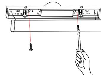
4. Press upward the cover and lock it with springs tightly which located into the fixture.
