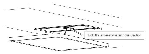
6. Align the aluminum frame notch of the lamp body to the U-shaped fold of the carrier board, and tighten the safety rope, and the aluminum frame notch will automatically align with the U-shaped fold of the carrier board. Place the lamp body flat on the mounting plane.
