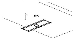
2. After the carrier plate is flattened to the ceiling, the four corner screws are locked.
