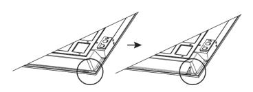
4 Rest the Luminaire on the T-Bar of the ceiling suspension system in the desired location.
