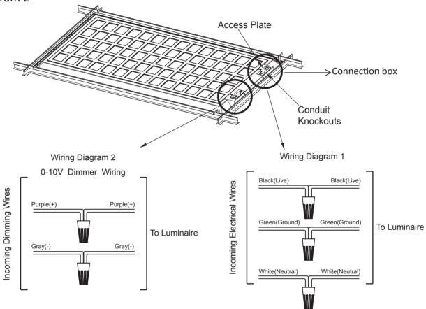
7 Check the wiring, make sure everything is correct. Recover the connection box. Then turn on power to light up the luminaire.
