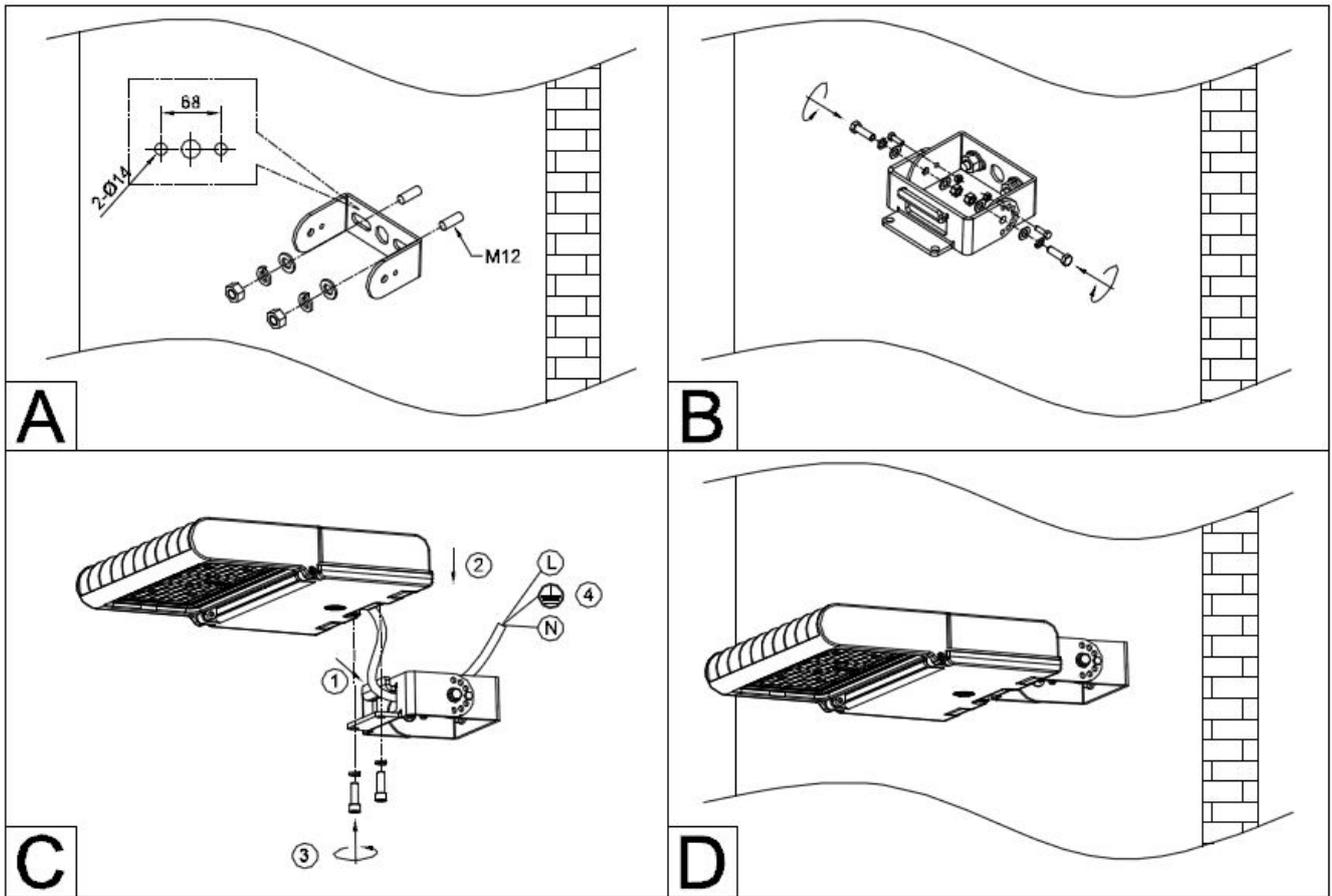
The mounting method of the straight arm is added to a wall mounted fixing plate, and the fixing plate is mounted on the wall, and the fixing plate is fixed by a nut.
