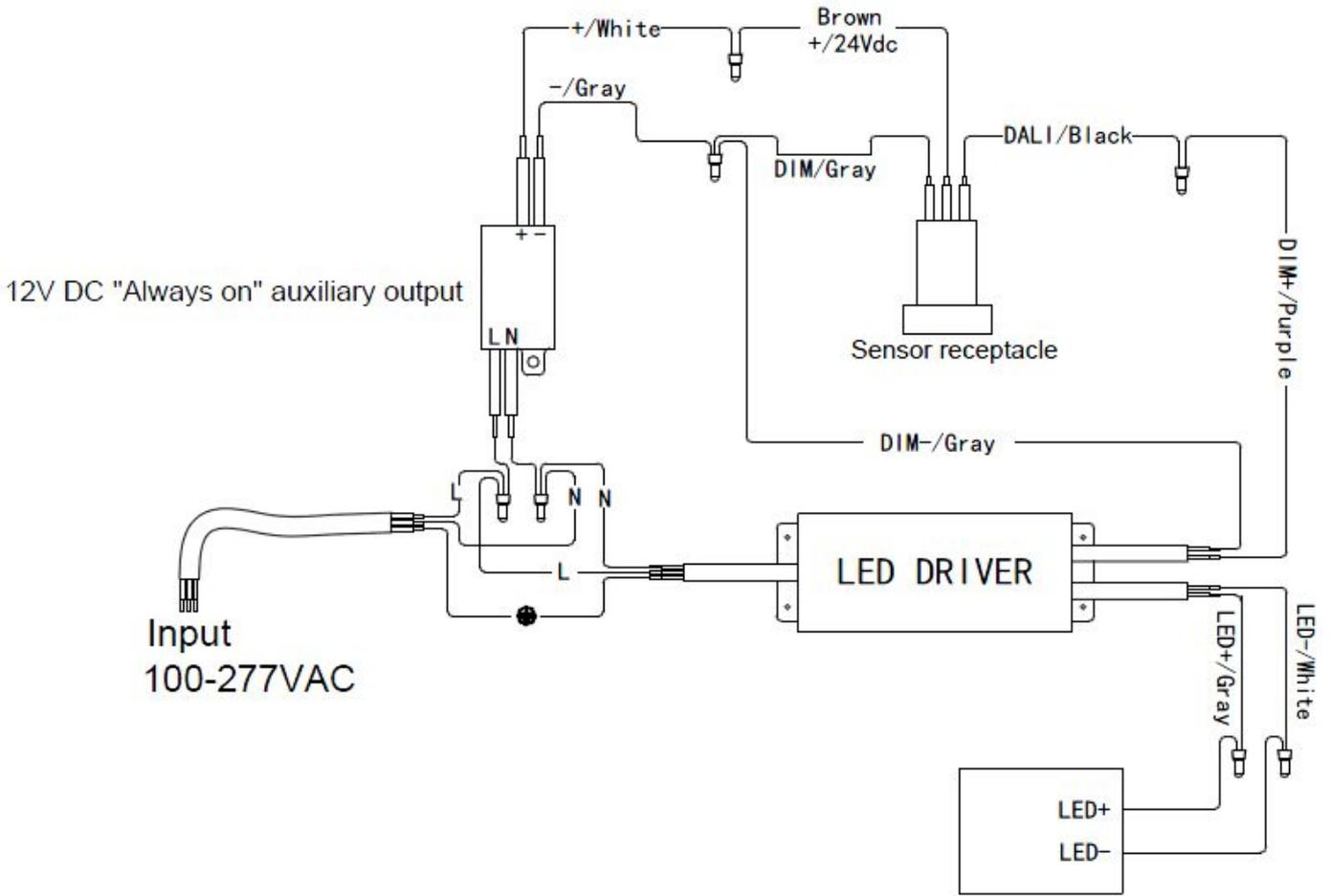
**Positions for Sensor and Photocell installed:**
