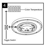
Connect the black wire to black (power) wire, white wire to white (neutral) wire with supplied wire connectors (BB). Tuck all wires into outlet box. Then secure the mounting screws tightly with screwdriver (not included).
