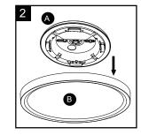
Pull out the source wires from the outlet box, thread them through the big hole of the ceiling pan (A).
