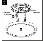
Attach the main body (B) to the ceiling pan (A) by aligning studs and slots, then turn it clockwise until it is locked in place.
