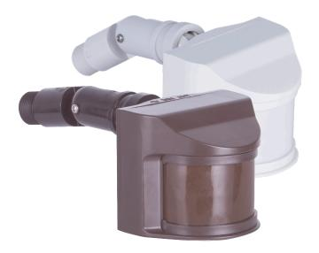
**SL-PIR** is a PIR sensor with 180° detection range and maximum 350W LED input. It is suitable for installation on flood lights as new installation or a replacement sensor. It has an adjustable mounting stem with setscrews. It is outdoor rated and made of tough polycarbonate material.
