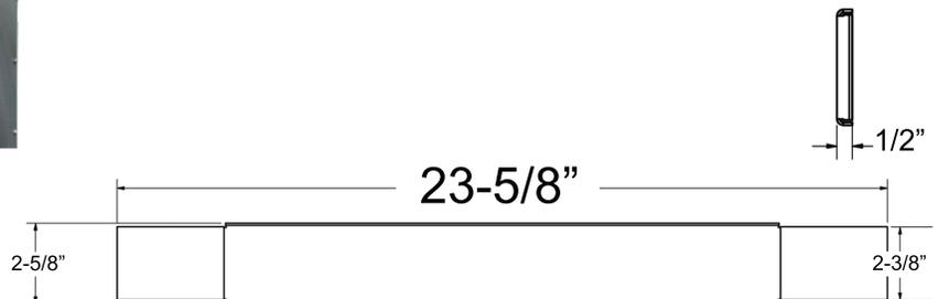
Cold-rolled Steel, Powder Coated White
