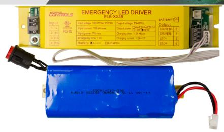
**ELB-2048** is a CEC-Compliant, UL-Listed and approved for field installation emergency lighting system for fixtures with **Isolated** drivers. For use with LED modules driven by a constant current source. The complete split system includes the EM driver, battery charger, battery, test switch with integrated indicator light.
