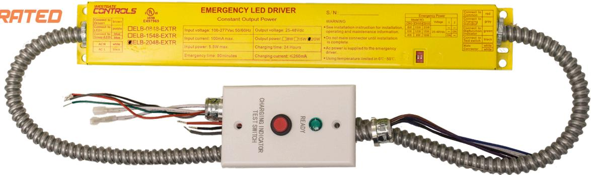
**ELB-2048-EXTR** is a CEC-Compliant, UL-Listed and approved for field installation emergency lighting system for fixtures with **Isolated** drivers. For use with LED modules driven by a constant current source. With an integrated battery and a test plate, it is a perfect choice for installation on panel lights and other commercial lights.
