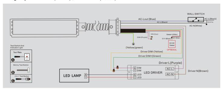
Wiring 3: For LED Driver With Input Power Less Than Emergency Output Power NON Dimmable LED Driver
