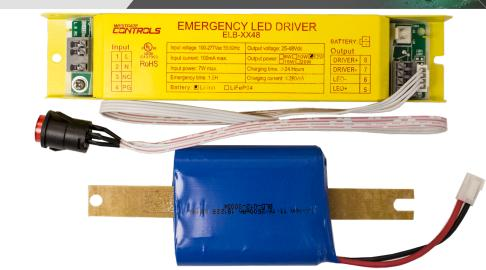
**ELB-1248** is a CEC-Compliant, UL-Listed and approved for field installation emergency lighting system for fixtures with **Isolated** drivers. For use with LED modules driven by a constant current source. The complete split system includes the EM driver, battery charger, battery, test switch with integrated indicator light.
