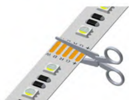
A1: Cut LED Strip along the cuttable mark
