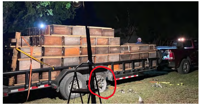
Blown trailer tire run down to the rim, Ouch!
