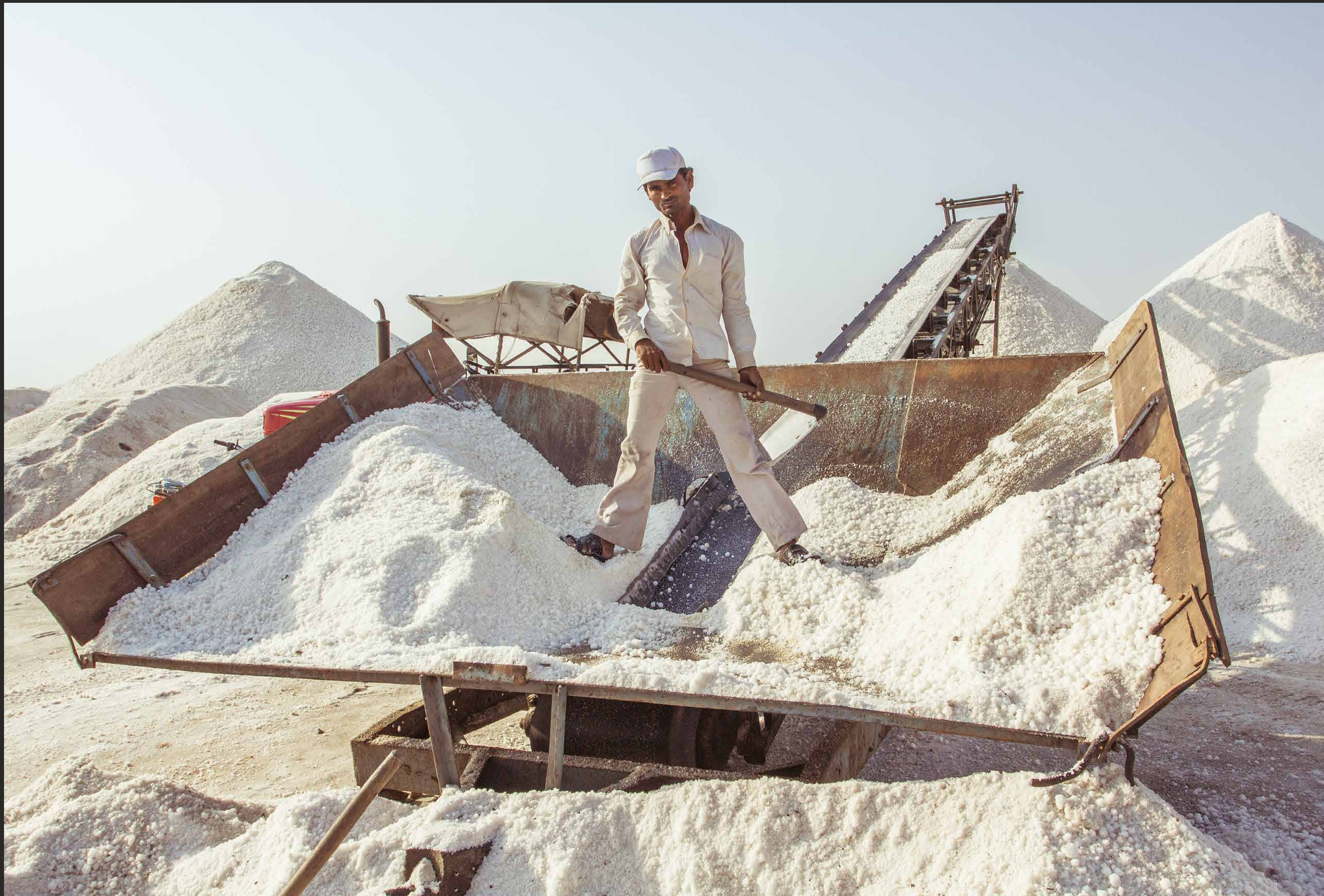
A worker feeding the salt hopper on the edge of the Rann for truck collection.
