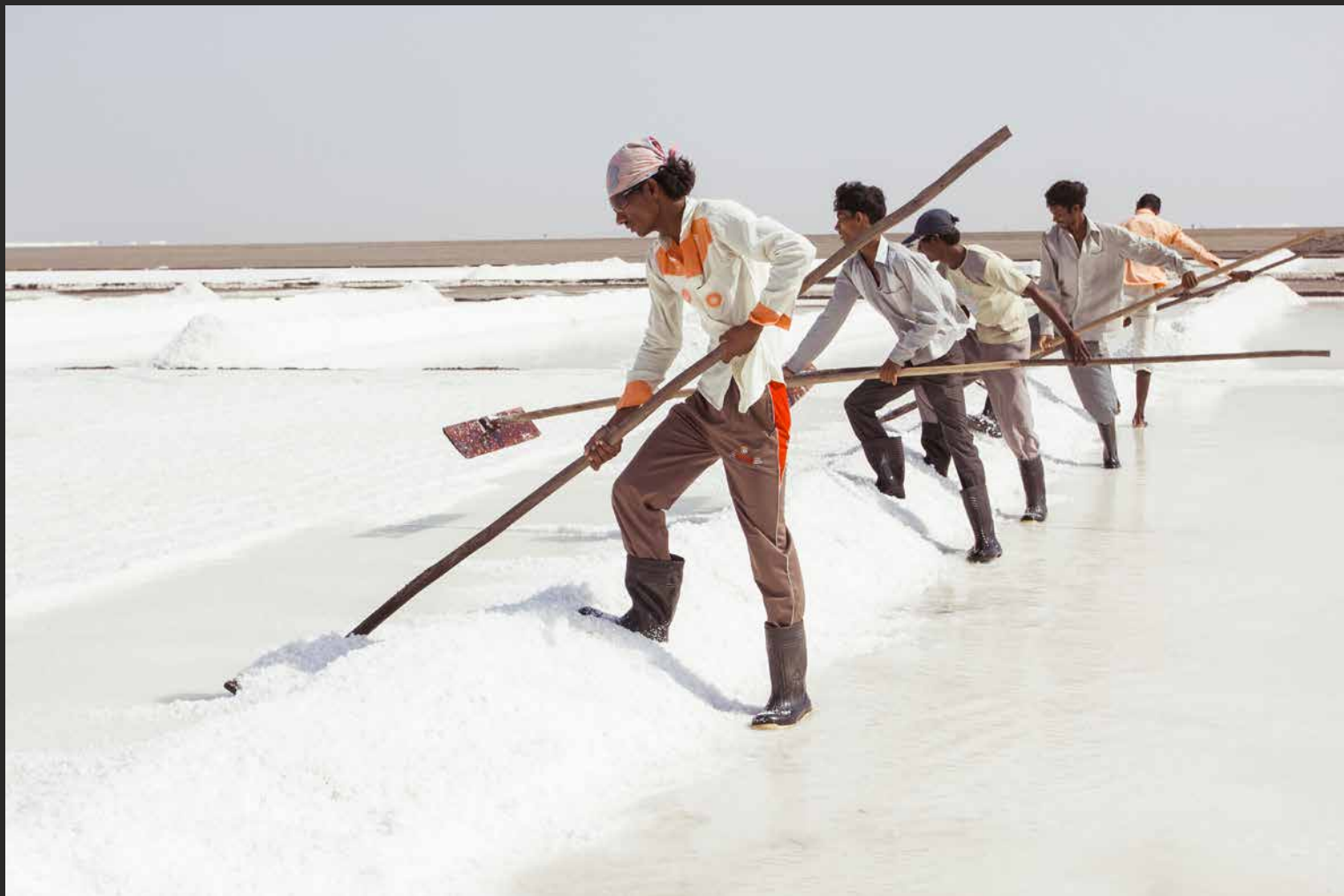
Workers starting the process of removing the salt crystals from the water in the salt pans.
