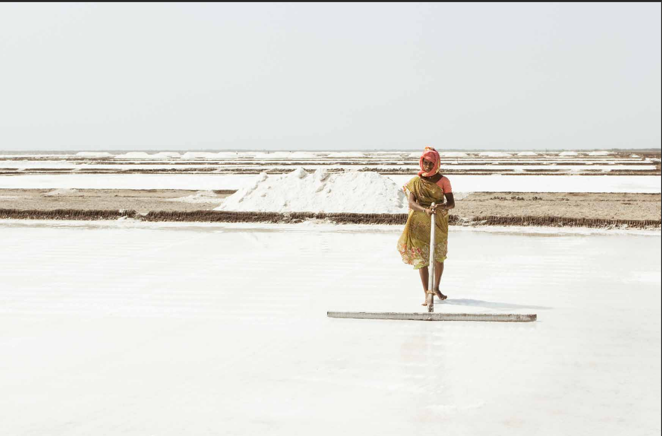
After the brine has been pumped from depth the water is raked and agitated over several days. Agariya workers use a wooden gantaras (rake) to allow evaporation and to encourage formation of the salt crystals.
