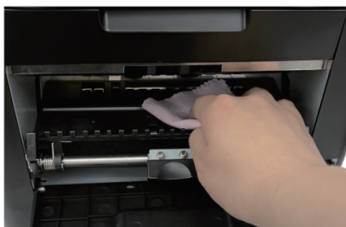
Clean the Lower CIS
