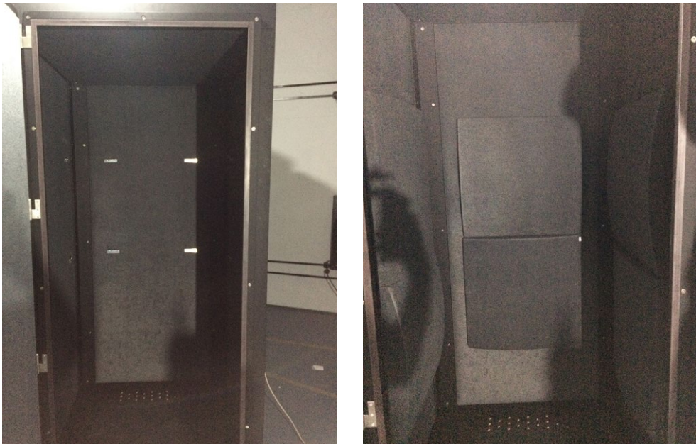
Figure 2 - VicBooth Ultra 1x1 - Left: without Cinema Round Premium inside (CL1); Right: with Cinema Round Premium inside (CL2).
