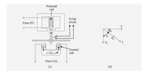
The interaction of fluxes  $\phi_1$  and  $\phi_2$  with the eddy currents induced in the disc produces a driving torque given by :
