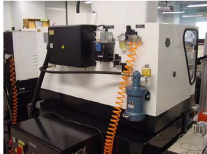
(b) Pneumatic system of an automatic machine
