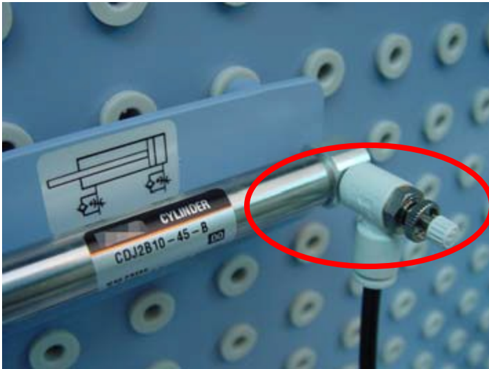
Fig. 14 (a) Flow control valve (b) Cross section (c) Pneumatic symbol
