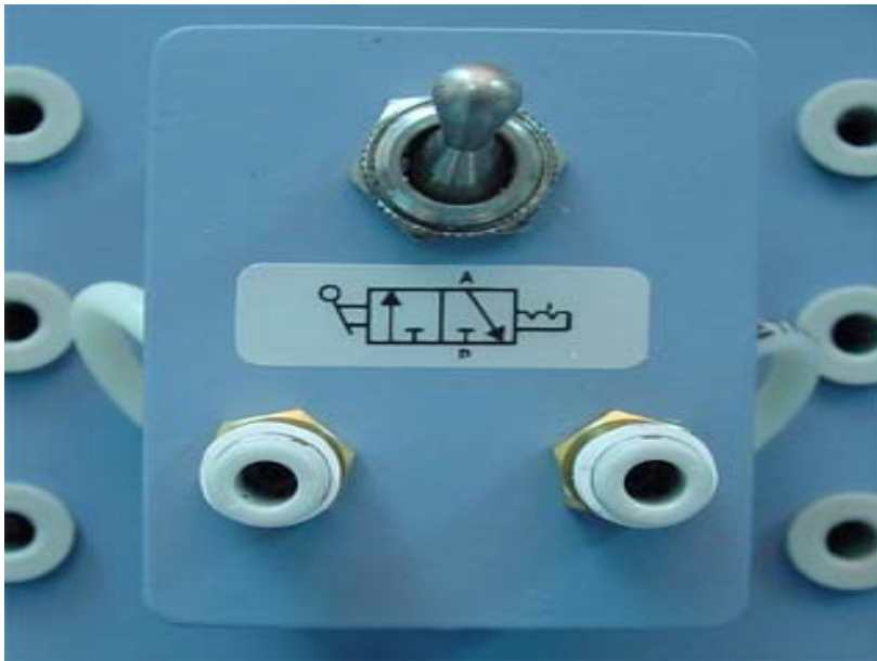
Fig. 10 (a) 3/2 directional control valve (b) Cross section
