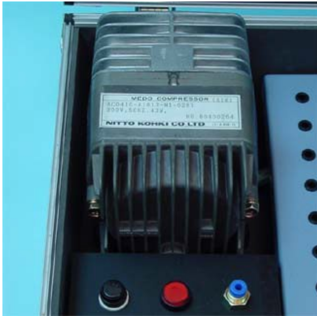
Fig 4 (a) Compressor used in schools (b) Compressor used in laboratories (c) Pneumatic symbol of compressor
