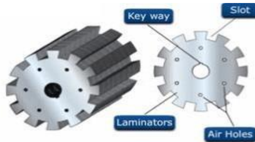
Figure 3: Armature of DC machine
