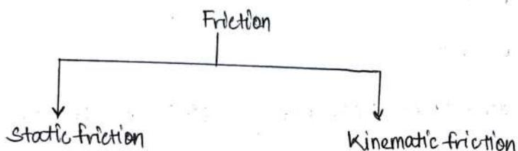
static friction - It is the friction between two surfaces (bodies), when they are at rest. (No motion) ( $f_s$ )
