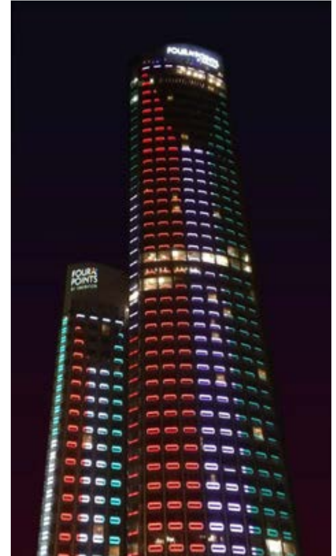
FOUR POINTS SHERATON, KUWAIT - PIXELFRAME supplied in custom lengths with die-cast end caps, corner pieces and end covers. Pixel mapped and controlled via DVI feed for image/animation/video playback.
