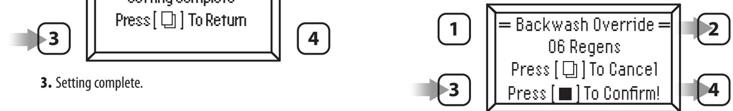
2. Press **buttons two (2) or four (4)** to select. Press **button three (3)** to Confirm.
