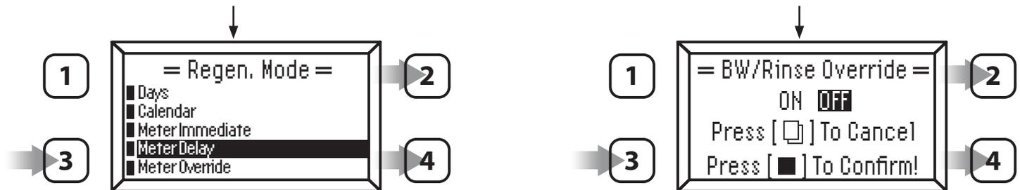
2. Press **buttons two (2) or four (4)** to select. Press **button three (3)** to Confirm.
