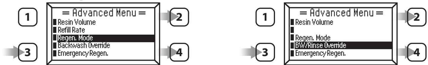
1. Press **buttons two (2) or four (4)** to select. Press **button three (3)** to Confirm.
