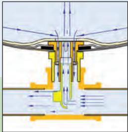
The patented **Flow-Thru™** connection features an innovative windvane insert that diverts system water into and, more importantly, out of the tank while the pump is running. This flushing action assures that the water in the tank remains fresh and eliminates the possibility of stagnant water during normal system operation.
