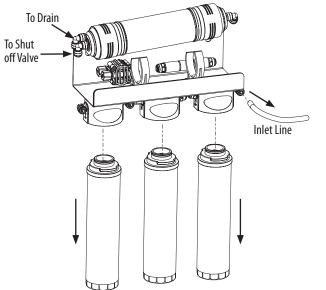
**2.** Disconnect all 4 cartridges and replace them with the empty sanitization cartridges included in this kit. Disconnect the inlet line from the system and drain excess water into a pail.
