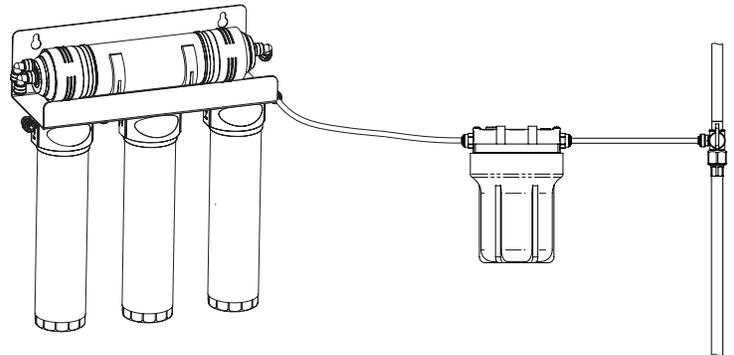
4. Using the tubing included in the kit, connect the sanitization cartridge between the adapter valve and the inlet port on the system.
