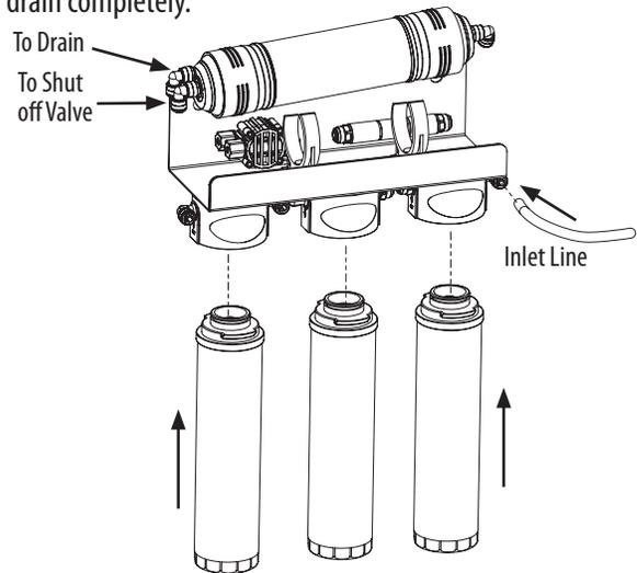
7. Disconnect the sanitization cartridge from the inlet line and system. Reconnect the inlet line to the system and replace cartridges on system.
