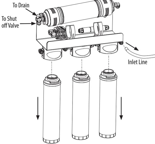
2. Disconnect all 4 cartridges and replace them with the empty sanitization cartridges included in this kit. Disconnect the inlet line from the system and drain excess water into a pail.
