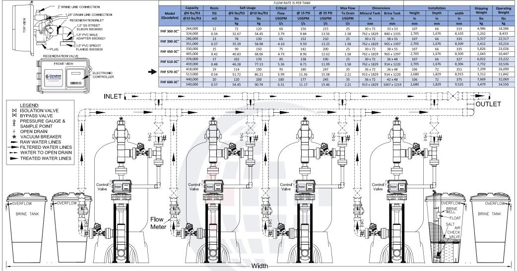
SOFTENER IS EQUIPPED WITH A 115 VOLT, ELECTRONIC SIDE MOUNTED REGENERATION CONTROL VALVE WITH 3"
